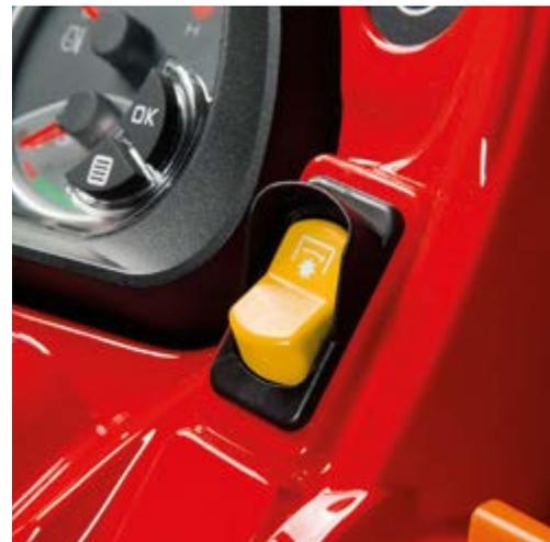
The two speed PTO: 540/540E rpm as standard, 540/540S rpm, 540/1000 rpm\* and synchronised with the gearbox speed. The ASAE 1 3/8 PTO shaft is the same for all speeds.
