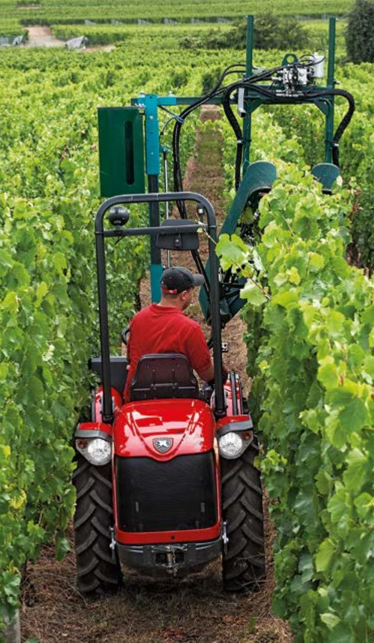
The tapered and racy design helps the tractor to maneuver in fields and increases operator visibility of the equipment and the surrounding terrain. The spacious driving position is easy to access and protects the operator. The operating station is suspended on **silent-block**, which absorb vibrations and dampen noise.
