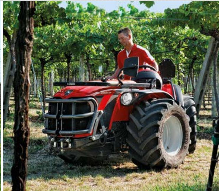
The short wheelbase and tight steering radius make the tractor extremely agile in crop rows. The smooth and sensitive hydroguide steering wheel assures precise maneuvering on steep slopes, in crossways movements, in narrow paths, among crop rows and in car parks. The hydraulic system of the hydroguide uses the Load Sensing system to obtain a constant flow of manoeuvrability independent of steering speed.
