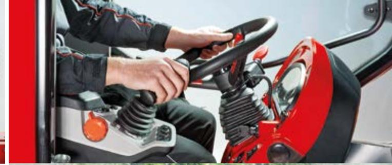
The lighting equipment, integrated into the mudguards, is comprised of reflecting parabolic optical assemblies, which offer a wide range of illumination covering the roadway, the equipment, and the surrounding field. The adjustable steering wheel allows any operator to find his ideal driving position. Maintenance is practical and fast thanks to the fact that the bonnet can be fully opened and the side panels and battery cover can be easily removed.
