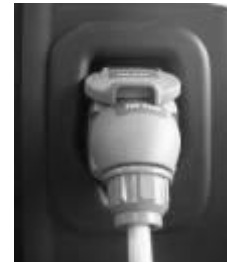
Position vertical after locking
