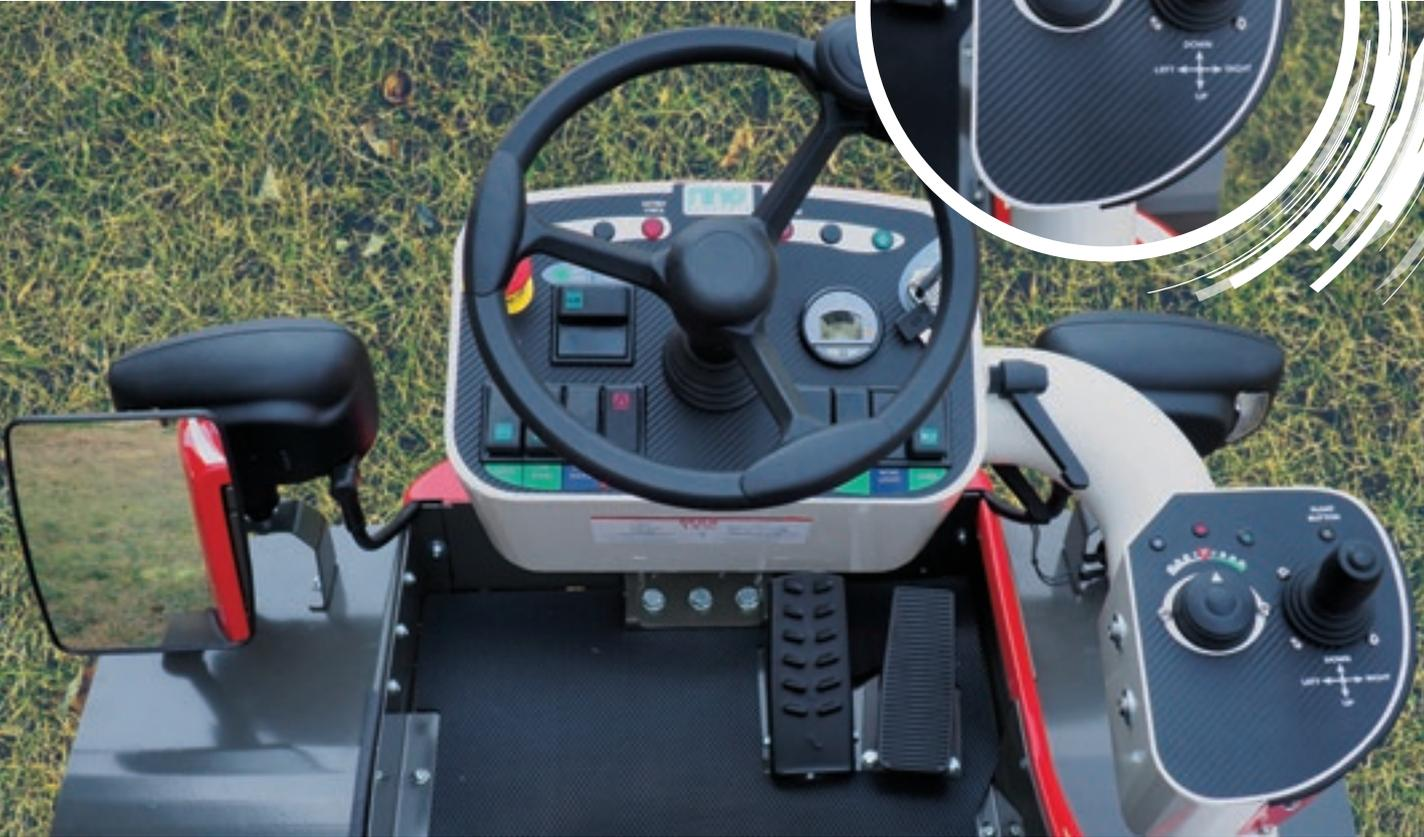
The control and information centre of the **RINO**<sup>®</sup> is designed for functionality with only essential elements. The principal data is shown on a display with the possibility to select the data required. The direction of travel and maximum speed are regulated by a rotary dial.
