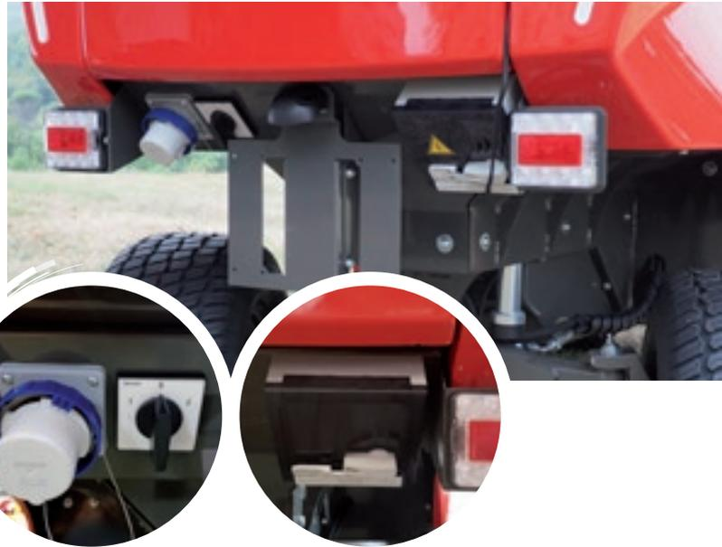
**RINO**® provides a “real” 18 kW (24cv) to two equal size electric motors, one to power the tractor and one to power the implements. It can be used with many power-hungry implements such as chippers, snow turbines, helicoidal lawn mowers.
