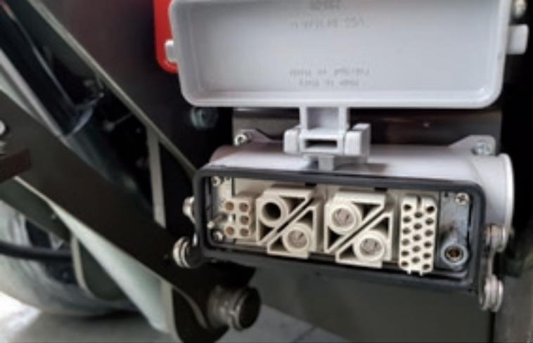
**Easy access to the electrical sockets for charging and for the 230 V, 50 Hz supply, which are located under the load bed.**
