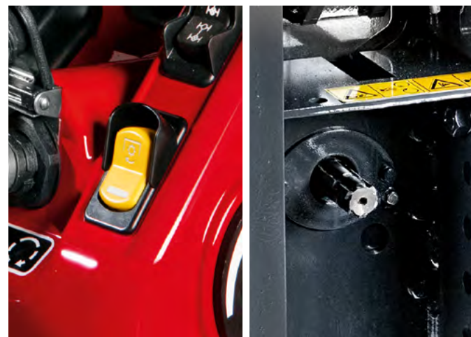
PTO with two speeds: 540/ 540E rpm (standard) with progressive electrohydraulic engagement; 540/ 1000 rpm* synchronised with the gearbox speed. A single 3/8 ASAE1 PTO shaft is used for all speeds.
