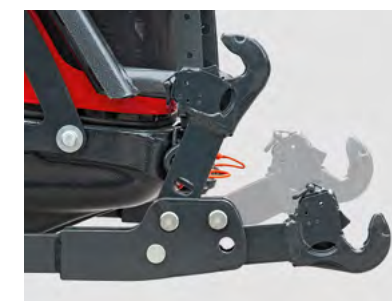
FRONT LIFT The front lift allows combined use of front and rear implements.
