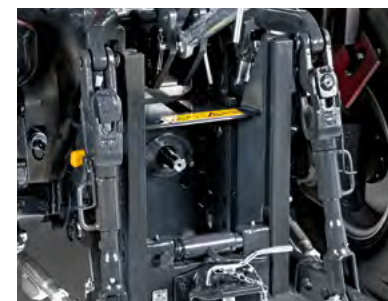
SLIDER HOOK Integrated into the rear lift, it gives the operator various options for the practical setting up of the tractor and the rapid alignment of the towed equipment.
