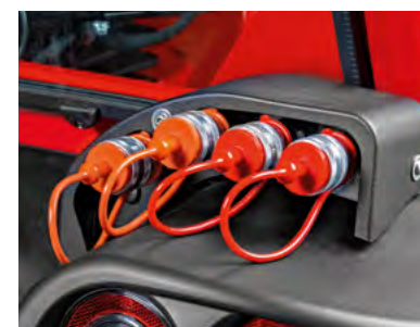
REAR QUICK COUPLERS 4 quick couplers as standard, hydraulically controlled from the driving position via the joystick + 4 additional mini-couplers.
