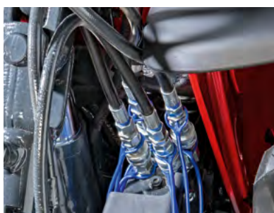
REAR QUICK COUPLERS 4 quick couplers as standard, hydraulically controlled from the driving position via the joystick + 4 additional mini-couplers.
