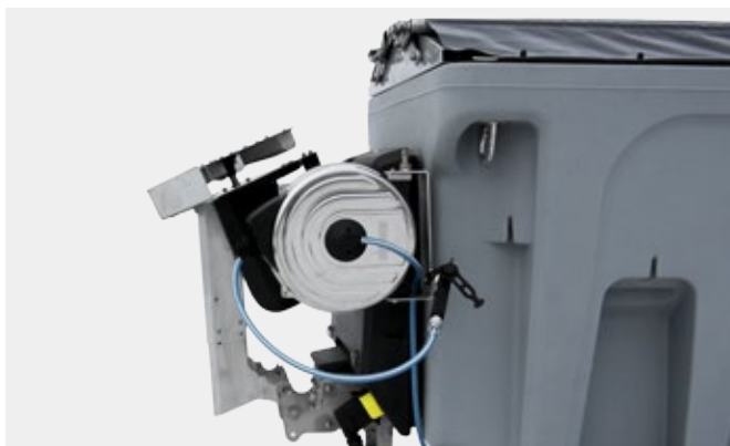
Stainless steel flip-up chute
