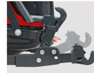
FRONT LIFT The front lift allows combined use of front and rear implements.
