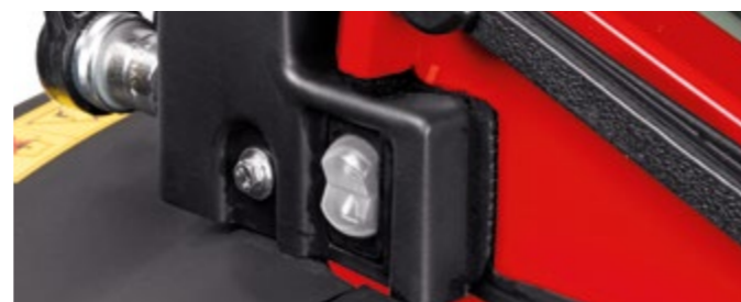
REAR LIFT CONTROL Positioned on the left and right rear mudguards; used to raise or lower the rear lift.
