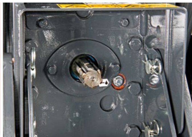
PTO With two speeds: 540/ 540E rpm (standard) with progressive electrohydraulic engagement; 540/ 1000 rpm* synchronised with the gearbox speed. A single 3/8 ASAE1 PTO shaft is used for all speeds.
