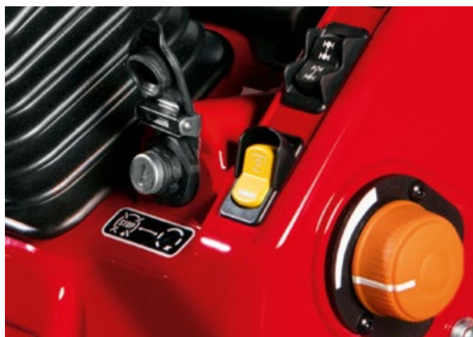
PTO With two speeds: 540/ 540E rpm (standard) with progressive electrohydraulic engagement; 540/ 1000 rpm* synchronised with the gearbox speed. A single 3/8 ASAE1 PTO shaft is used for all speeds.
