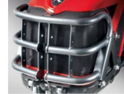
BULLBAR Tubular steel guard protecting the bodywork; integrates the third-point for the front lift.
