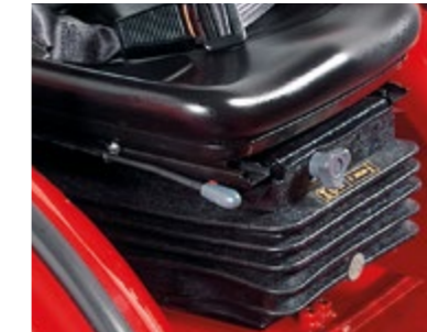
PNEUMATIC SEAT Latest generation with air springs.
