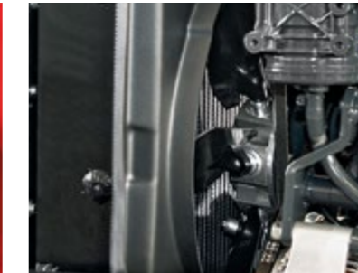
ACS (Air Clean System) Engine cooling fan with air flow reversal. Reduces the need for cleaning the front grille, ensuring more constant engine cooling.
