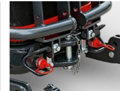
FRONT QUICK COUPLERS Hydraulic front lift complete with 3-point linkage + 1 replicated front double-acting remote (2 front quick couplers).
