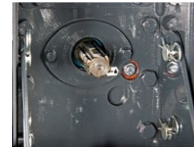
PTO Gearbox with PTO 540-1000 rpm.
