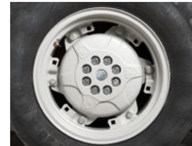
REAR CAST IRON WHEEL FLANGES Flanges that increase the weight of the tractor at the rear.
