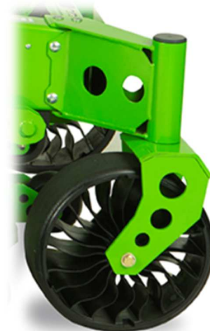
Front airless Michelin X Tweels® Turf 13"
