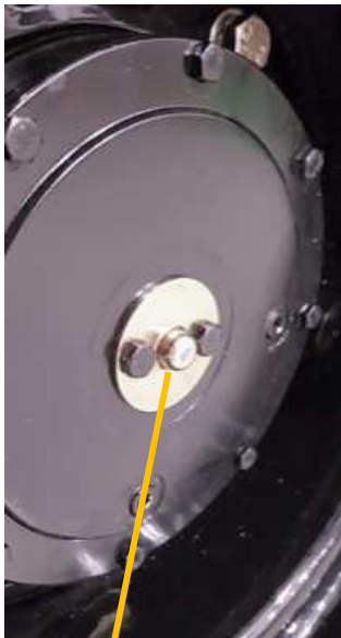
BUTTON PUSHED OUT BRAKE ENGAGED
