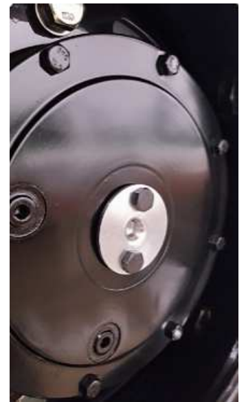
BUTTON PUSHED IN BRAKE DISENGAGED
