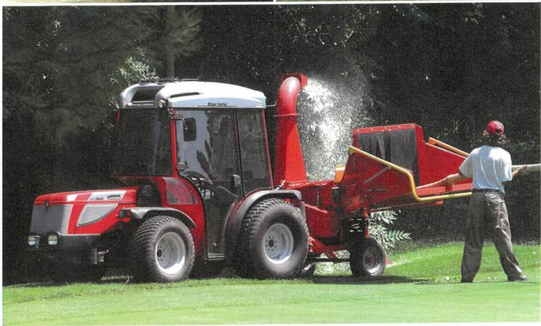
The hydrostatic transmission grants unbeatable operative practicality during rapid forward and backward movements in quick succession. The reverser lever allows to change quickly and easily the drive direction. It is fitted with the **speed-fix** device, an authentic specialist when executing activities that require constant forward speeds.
