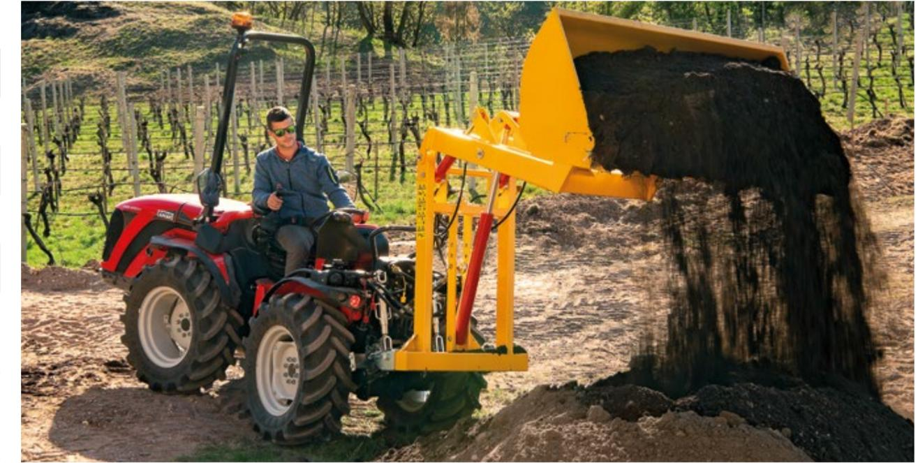
The *Load Sensing* hydraulic system raises the application suitability of the latest generation of complex implements to all models in the range. Increased hydraulic flow rates with adjustable continuous flows allow for maximum control in the management of the most demanding implements, such as in-row tillers or foliage pruning machines. In addition, the Tora (reversible) can be configured with the new multifunctional *Hydraulic Remote Control*\*.
