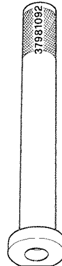
11 - Driver for the mounting of the axle shaft bearings.
